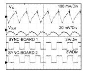
Figure 55. Output voltage ripple of two modules with synchronization clocks 180 degrees out of phase
