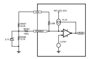
Figure 50. Enable input detail
