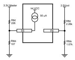
Figure 51. Tracking option input detail
