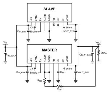
Figure 53. Current Sharing Example Schematic
