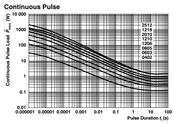
Maximum pulse load, continuous pulses; applicable if  $\overline{P} \le P(\vartheta_{amb})$  and  $\hat{U} \le \hat{U}_{max}$ ; for permissible resistance change equivalent to 8000 h operation
