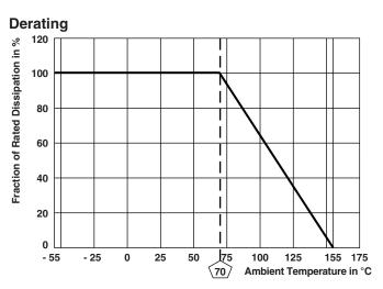
Pulse Proof, High Power Thick Film Chip Resistors
