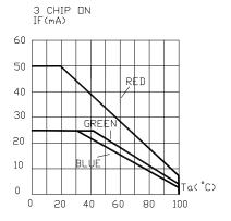
MAXIMUM FORWARD DC CURRENT VS, AMBIENT TEMPERATURE.
