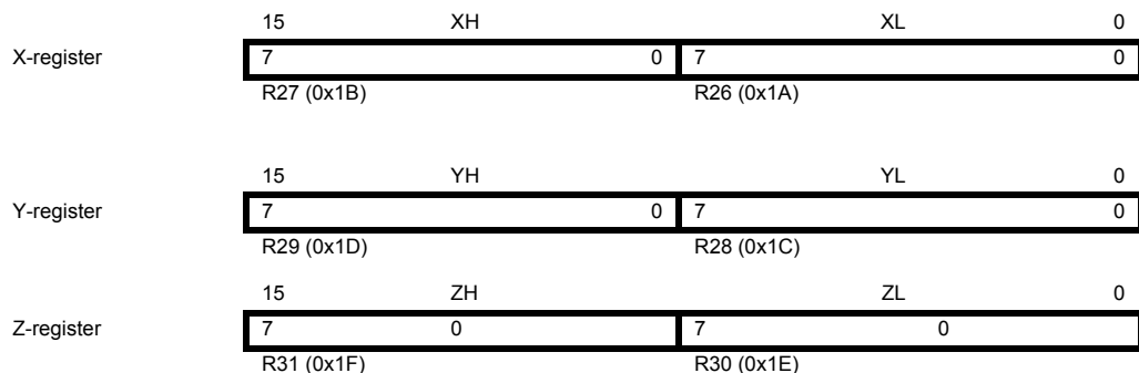
Figure 4-3. The X-, Y-, and Z-registers
