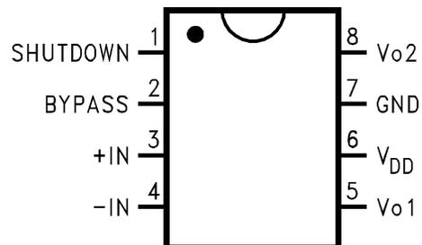
**Figure 2. Small Outline and PDIP Package-Top View**
