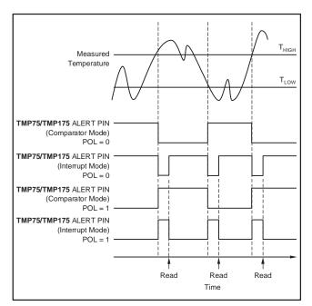
Figure 3. Output Transfer Function Diagrams
