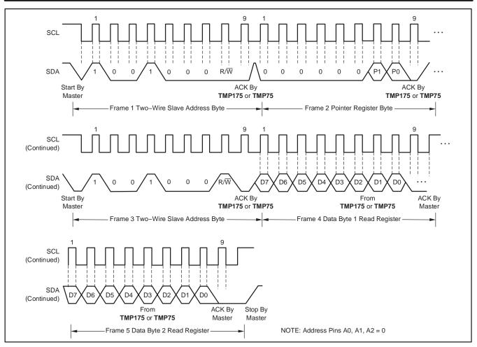
Figure 7. Two-Wire Timing Diagram for Read Word Format
