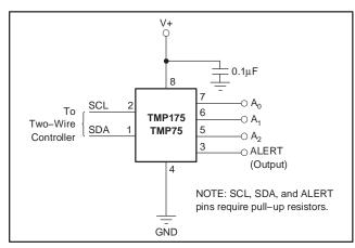
Figure 1. Typical Connections of the TMP175 and TMP75
