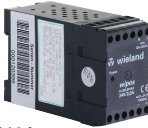
24 V / 2 A Primary switch-mode regulator CE; Approvals: UL, CSA and pending 45 x 72 x 105
