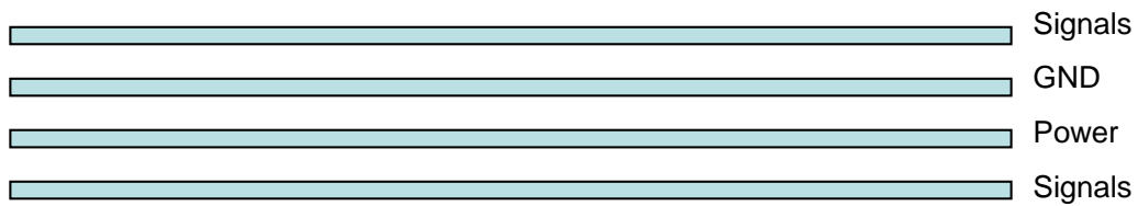
Figure 12: Typical 4-layer PCB construction
